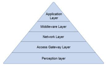
Fig. 2. Five-layer architecture of the IoT.
